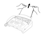
**2** Open the top cover by lifting the lever on the right side of the top cover.
